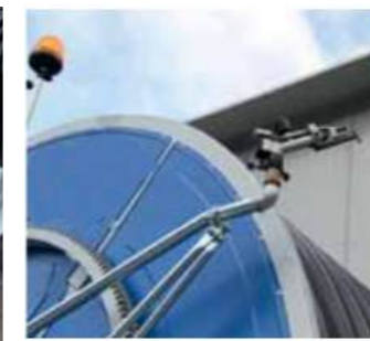
Second sprinkler on the machine frame
