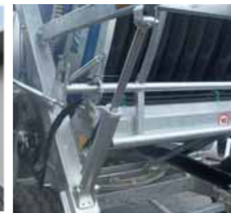
Trolley lifting with hydraulic cylinders
