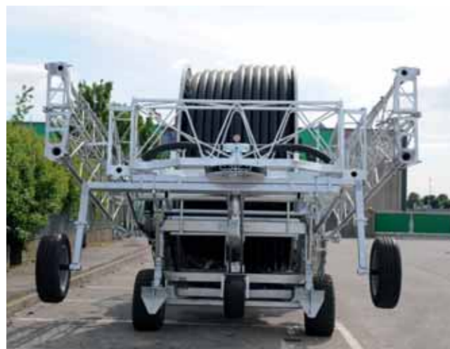
Turbocar with standard Spraying boom
