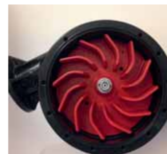
Turbine PLASCOAT painting
