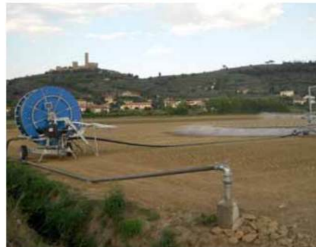
Turbocar with folding Spraying boom
