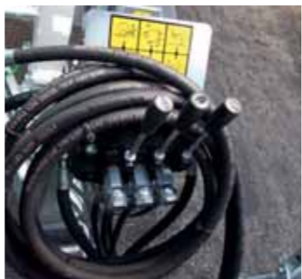
Distributor with fast clutch hoses
