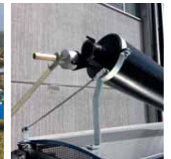
Self-priming device vacuum operated
