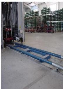
A fixed, pipe-rail weighing scale, including or excluding automatic cart recognition
