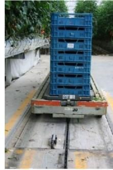
A fixed, countersunk weighing scale, including or excluding automatic cart recognition
