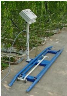
Mobile weighing scale, including or excluding automatic cart recognition
