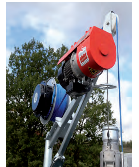
Electric winch for up-lift of electric pump
