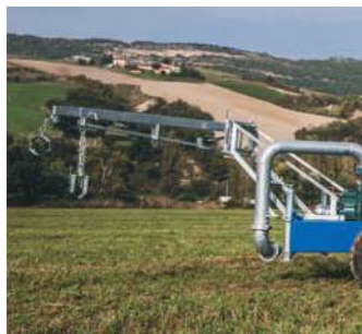
Arm-holder to lift up the suction pipe
