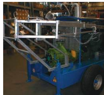
Hydraulic Arm-holder to lift up the suction
