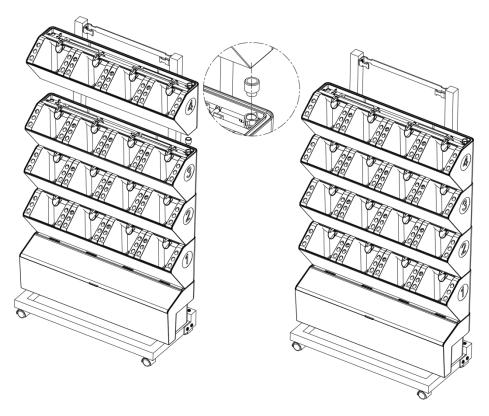
6) Install the 5th layer of the flower box, and put two end plugs into the holes as shown in the figure.
