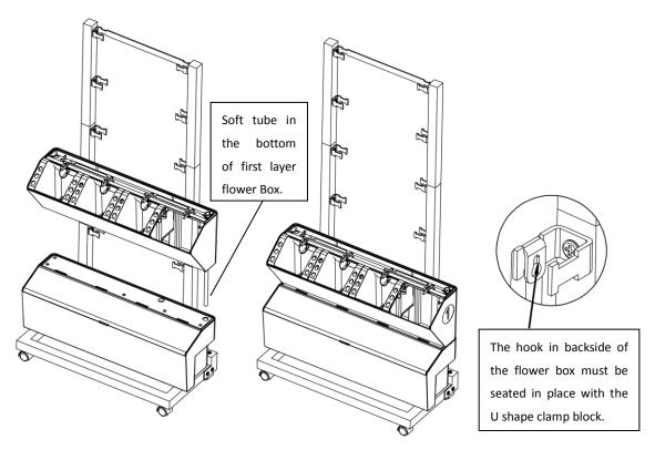
Connect the water pipe of the flower box with bottom water tank section, and make sure buckle fastened.
