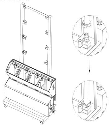
Install second layer of the flower box as shown in the figure(be sure the seal is put at right position).
